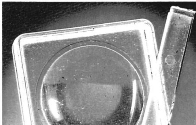
Figure 9.39 Dark spots due to thermal damage
