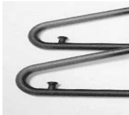
Figure 10.16 Marbling effect on a moulding
